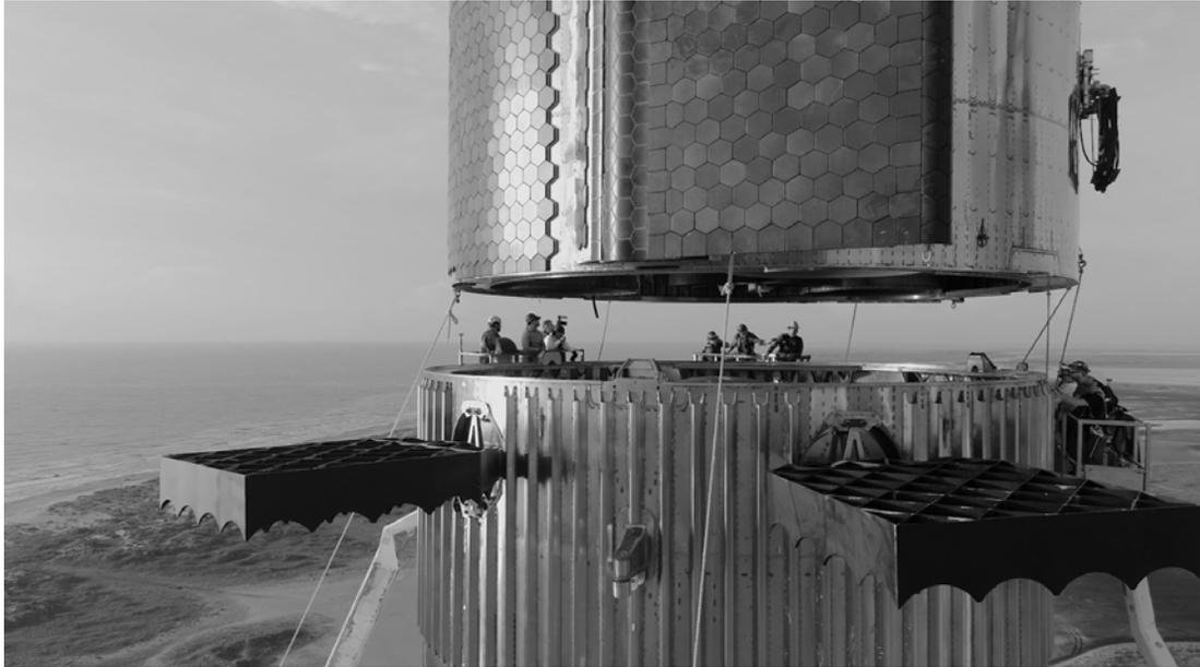
Figure 9: Starship being mated with its Super Heavy Stack (Credit: SpaceX)
